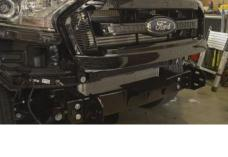
33. Fit the new bash plate over the bullbar and mount using the supplied nuts and bolts.
